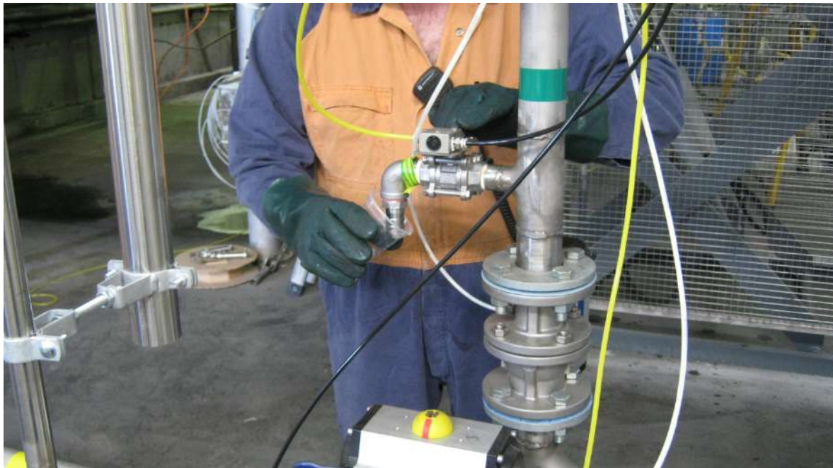
Photo 3: New automated sampling system with built-in safety mechanisms
